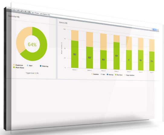
Visual display of water level in the plant root zone for each irrigation station.
